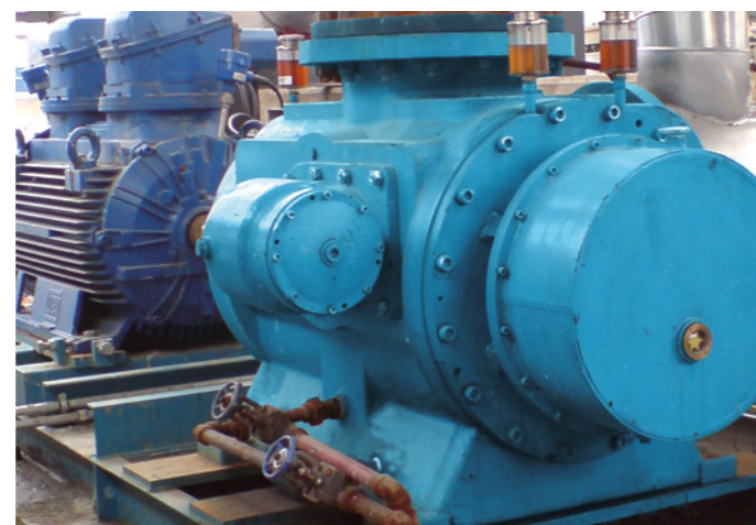
Crude oil is circulated using the L2, L3 and L4 pump series to avoid separation, to maintain temperature and to flush system pipework.
